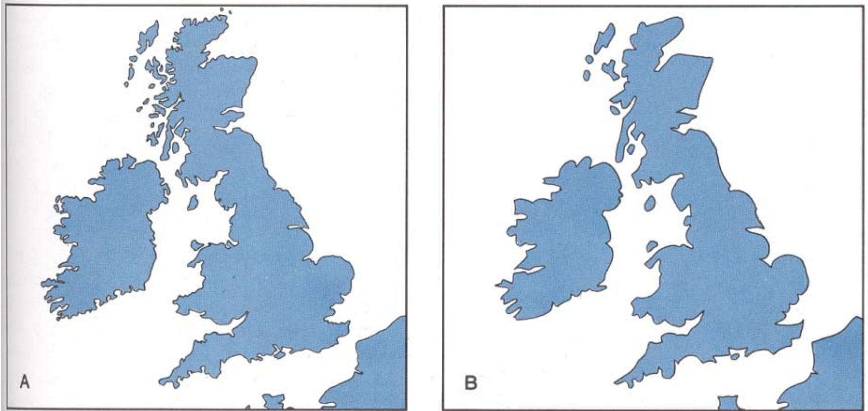
Figure 24.6 Two representations of Great Britain and Ireland at the scale of about 1:15,000,000. The map on the left (A) is simplified to fit the scale and is suitable for a reference map intended to give the impression of detailed precision. The map on the right (B) is a diagrammatic generalization suitable as a base on which to display thematic data. Note that (B) captures basic shapes, which tend to be masked by the detail in (A).
